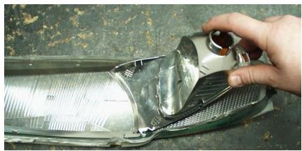
With this removed the orange lens can be removed with a small screwdriver or by popping it out using a finger pushed through the hole for the bulb.
