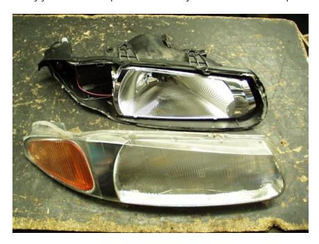
The indicator reflector and orange lens are clipped into the main lens section, to remove it unclip the corner marked 1,release the end marked 2 and finally release the hooked end marked 3.
