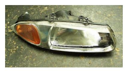
You will start separating the two halves starting at the indicator end of the assembly...but FIRST remove the small white plastic clip arrowed.
