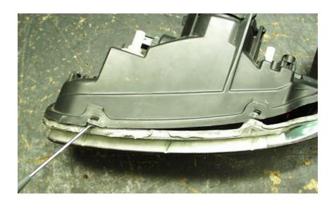
There are five clips in total, two on top, two on the bottom and one on the edge at the headlight end.
