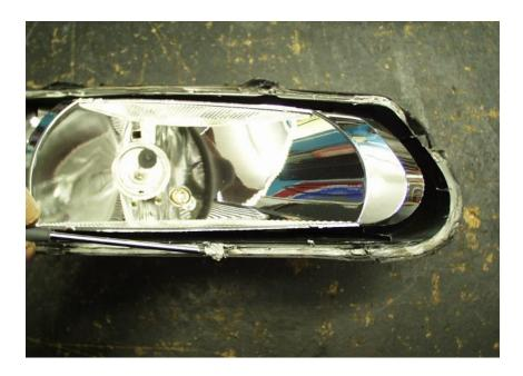
Use a silicone mastic to replace the original grey sealant, preferably a non acetic type such as RITO. There is no need to fill the groove right to the top as it will squeeze out everywhere when the two halves are reassembled. Fill the groove about one third the way up.
