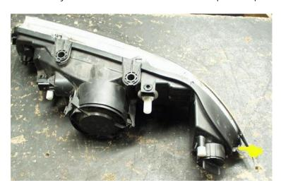
The two halves are held with clips moulded into the black section, also a bead of mastic is used to provide a watertight seal.
